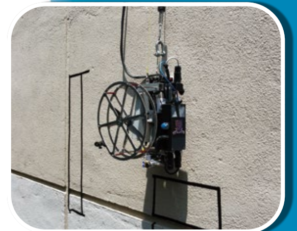
Hammer tapping robot working on the external wall
