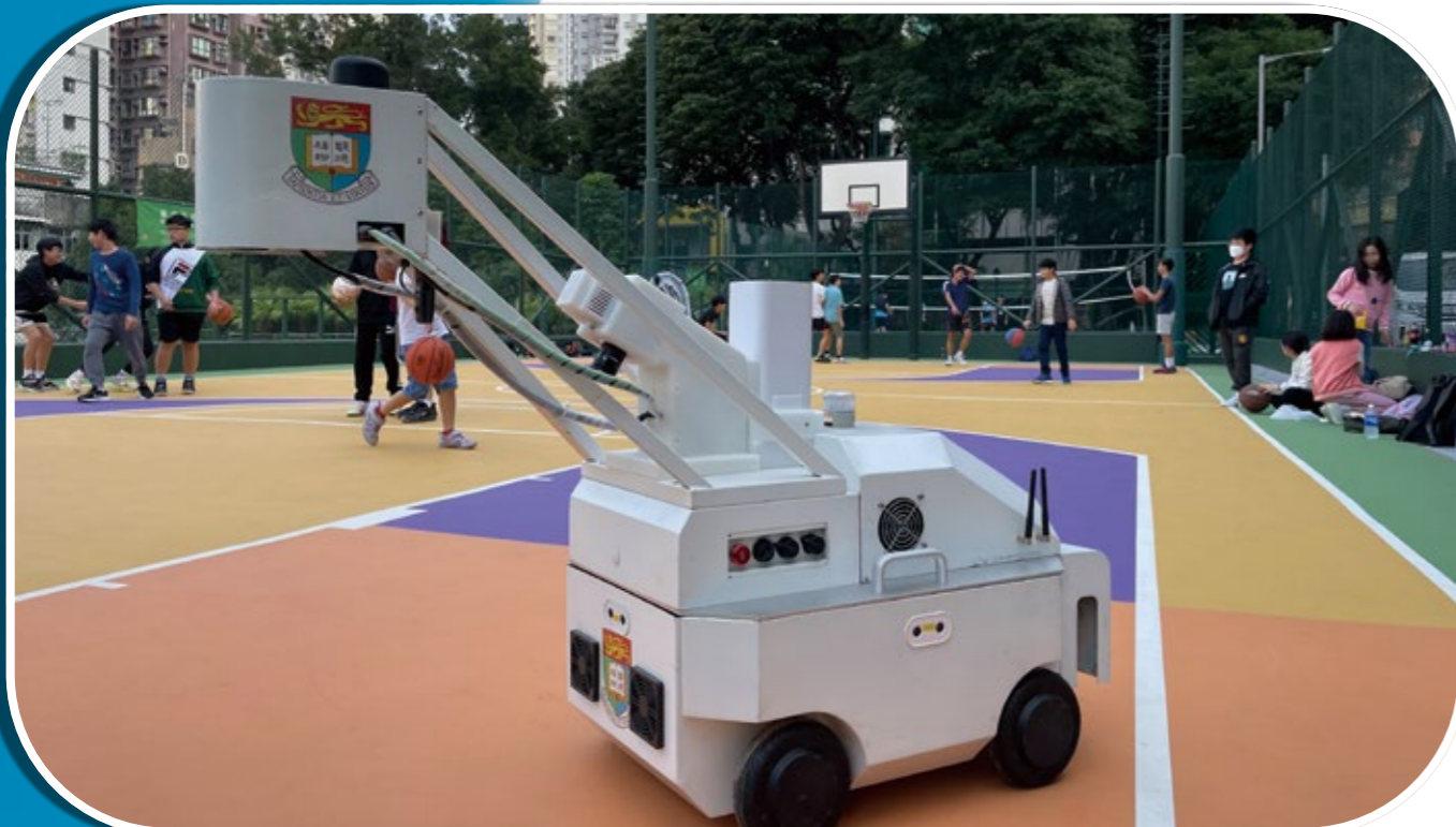
Sports Flooring Inspection Robot to assist in quality check of resurfacing works in Blake Garden
