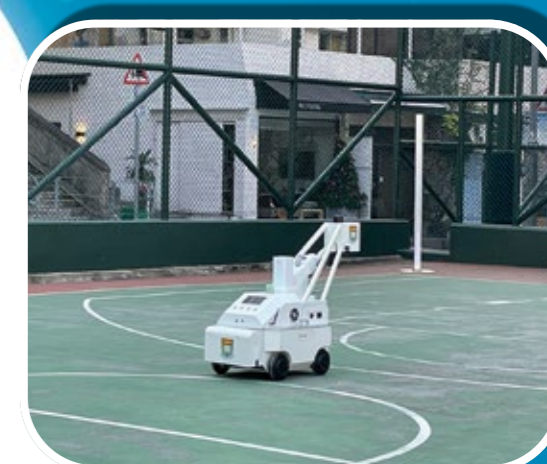
Automated scanning of the ball court floor surface to identify defects
